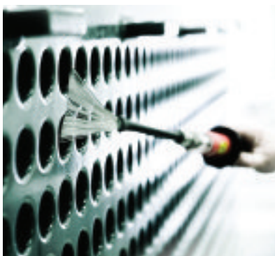
A tube plate coated by Acccoat to be used at a refinery using the Topsøe SNOX™ technology
